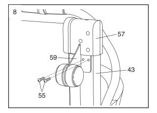
9. Make sure that all parts are properly tightened before you use the Incline Trainer. Keep the included allen wrench in a secure place. The allen wrench is used to adjust the walking belt (see page 31). To protect the floor or carpet from damage, place a mat under the Incline Trainer.
